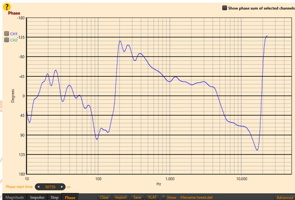
Picture 50: phase plot after start time adjustment
