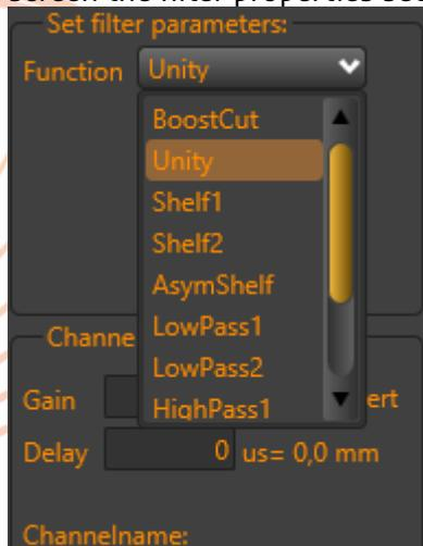
Picture 21: Select the filter object function
