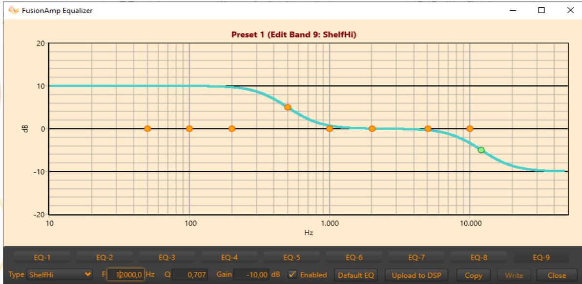
Picture 57: Equalizer screen, band 9 selected and frequency changed to 12kHz
